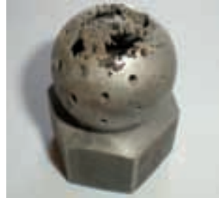
Fig. 1: Chemical corrosion of a spray ball
