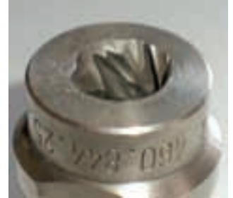
Fig. 2: Wear of a full cone nozzle
