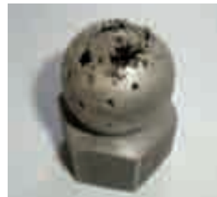
Figure 18: Chemical corrosion of a spray ball
