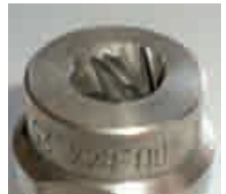
Figure 19: Wear of a full cone nozzle
